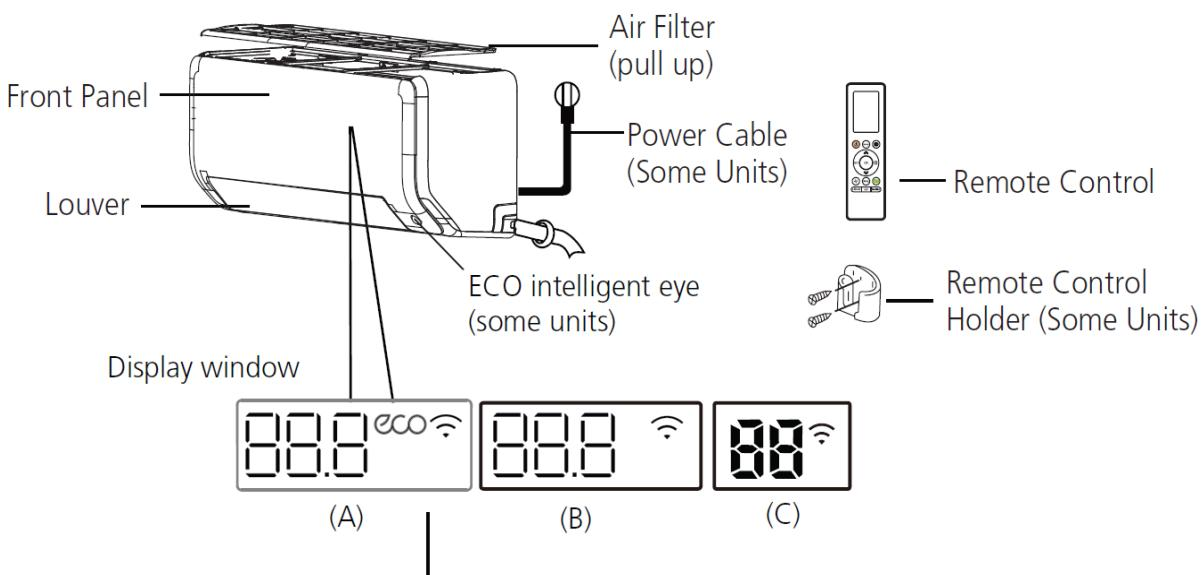
“**88.8**” “**88**” Displays temperature, operation feature and Error codes:
